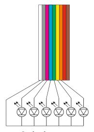
**Ex2:CommonCathode**on the SIDE737 board (if any) set the jumper in KC position for common cathode led configuration
