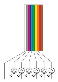
**Ex1:Common Anode** set the jumper in AC position for common anode led configuration
